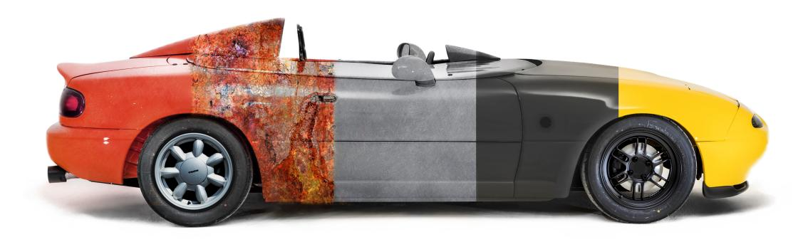
Each original donor chassis undergoes a **complete restoration**, consisting in four main processes: 1) Pyrolytic paint stripping: heat is applicated without the use of a flame, in a process following a specific progression of times and temperatures. This allows a complete cleaning of the shell, removing all residues of paint and sealing glues.
